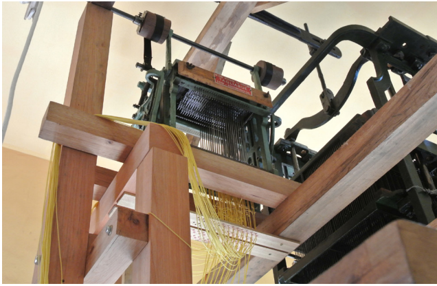
Donated Italian-made 104 hook 'Giacomino' Jacquard loom installed at the Peers atelier. © J Holyoke 2015.
